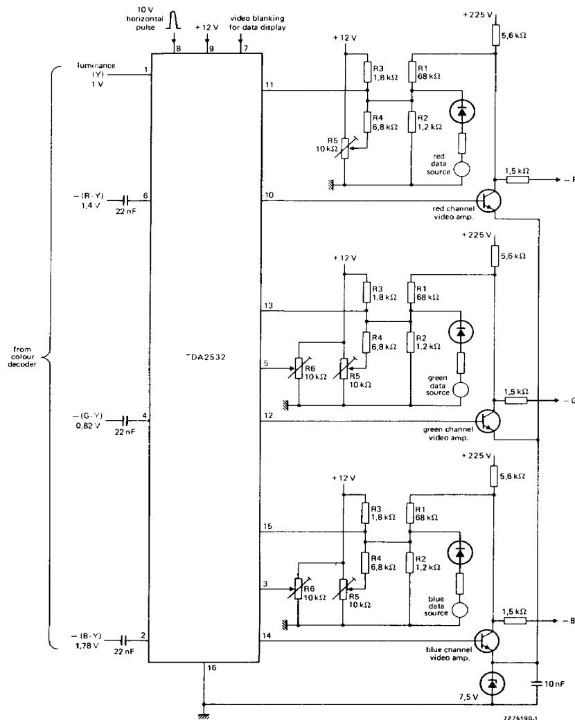
R5 = clamping level adjustment (70 V to 170 V); R6 = gain adjustment (65 to 140).
