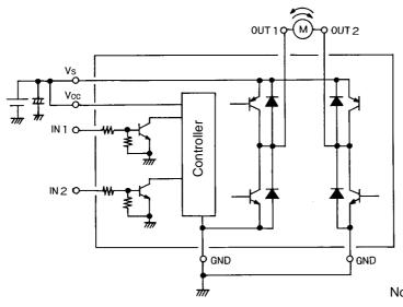
Note: When using the same power supply for  $V_S$  and  $V_{CC}$ , short the  $V_{CC}$  and  $V_S$  pins to each other or insert a capacitor in the  $V_{CC}$  line.
