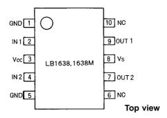
Note: both ground pins must be grounded.
