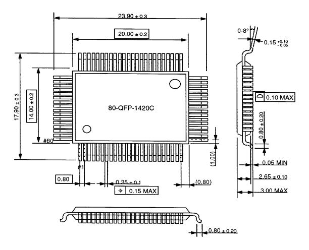
NOTE: Dimensions are in millimeters.
