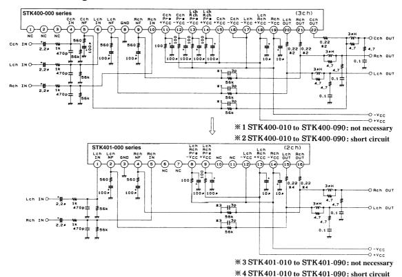
Unit (resistance:  $\Omega$ , capacitance: F)
