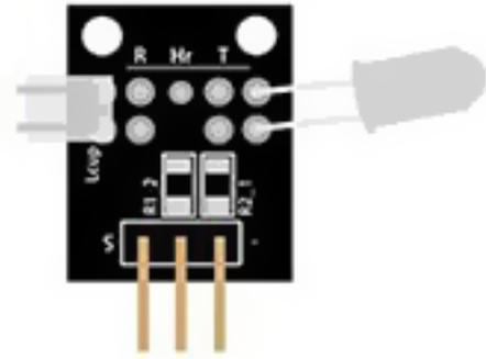
Pulse monitor works as follows: The LED is the light side of the finger, and photo transistor on the other side of the finger, photo transistor used to obtain the flux emitted, when the blood pressure pulse by the finger when the resistance of the photo transistor will be slightly changed.
