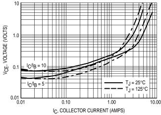
Figure 4. Collector–Emitter Saturation Voltage
