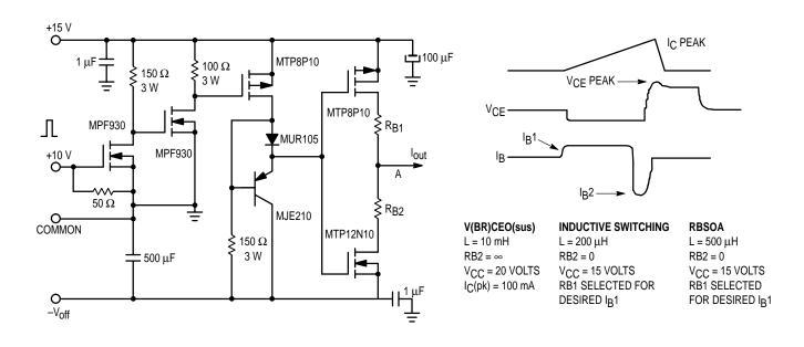
Table 1. Inductive Load Switching Drive Circuit
