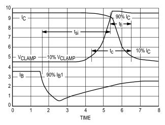
Figure 19. Inductive Switching Measurements
