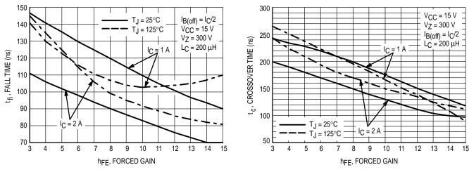
Figure 13. Inductive Fall Time, t<sub>fi</sub>(hFE)
