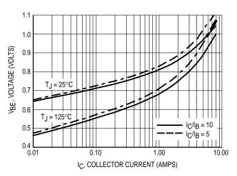
Figure 5. Base–Emitter Saturation Region
