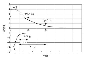
Figure 18. Dynamic Saturation Voltage Measurements
