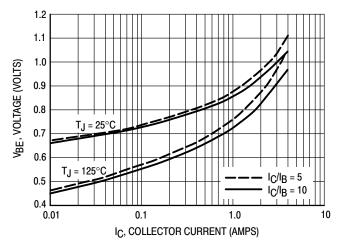
Figure 5. Base-Emitter Saturation Region
