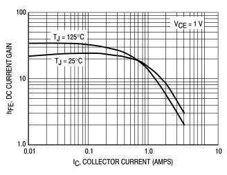
Figure 1. DC Current Gain at 1 Volt
