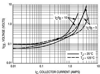
Figure 4. Collector-Emitter Saturation Voltage
