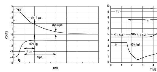
Figure 18. Dynamic Saturation Voltage Measurements
