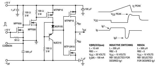
**Table 1. Inductive Load Switching Drive Circuit**
