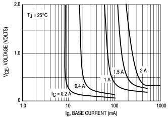
Figure 3. Collector Saturation Region
