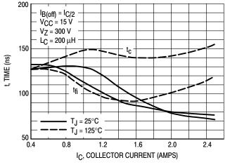
Figure 11. Inductive Switching,  $t_C$  and  $t_{fi}$   $I_C/I_B = 5$
