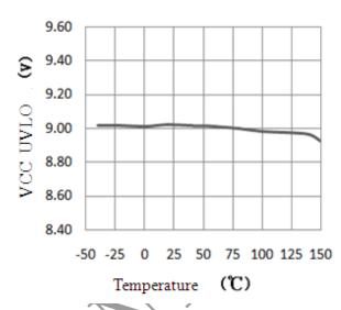
Turn off threshold VS. Temperature
