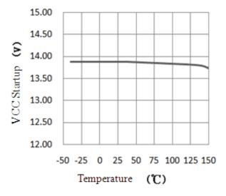
Turn on threshold VS. Temperature
