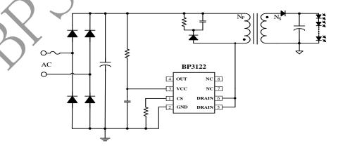
Figure 1. Typical application circuit for BP3122
